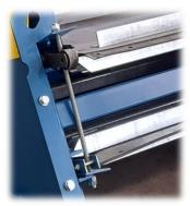
Threaded rods are used to secure the belt against movement during transport and handling, which must be removed before connecting the belt.
