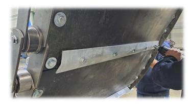
The belt begins to be installed in the area of the mounting side (upper route) and/or in the area of the tensioning head (lower or upper route). It always depends on the spatial possibilities of a specific installation.
